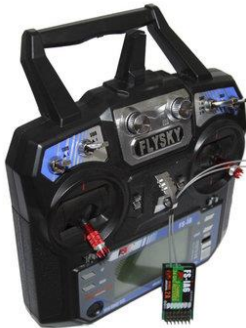
Fig12: Flysky Transmitter and Receiver
